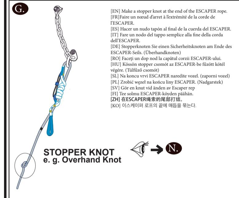
[EN] Make a stopper knot at the end of the ESCAPER rope.
